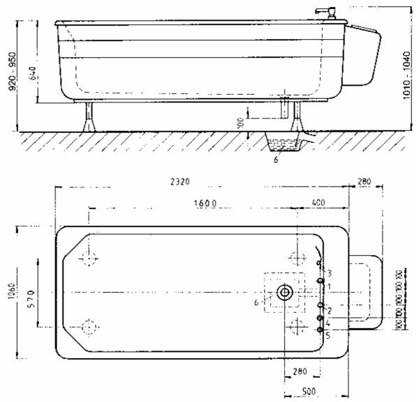
Combinationappliance model Freiburg type UW GI CO<sub>2</sub> 2000 AC part-no. AU1185
